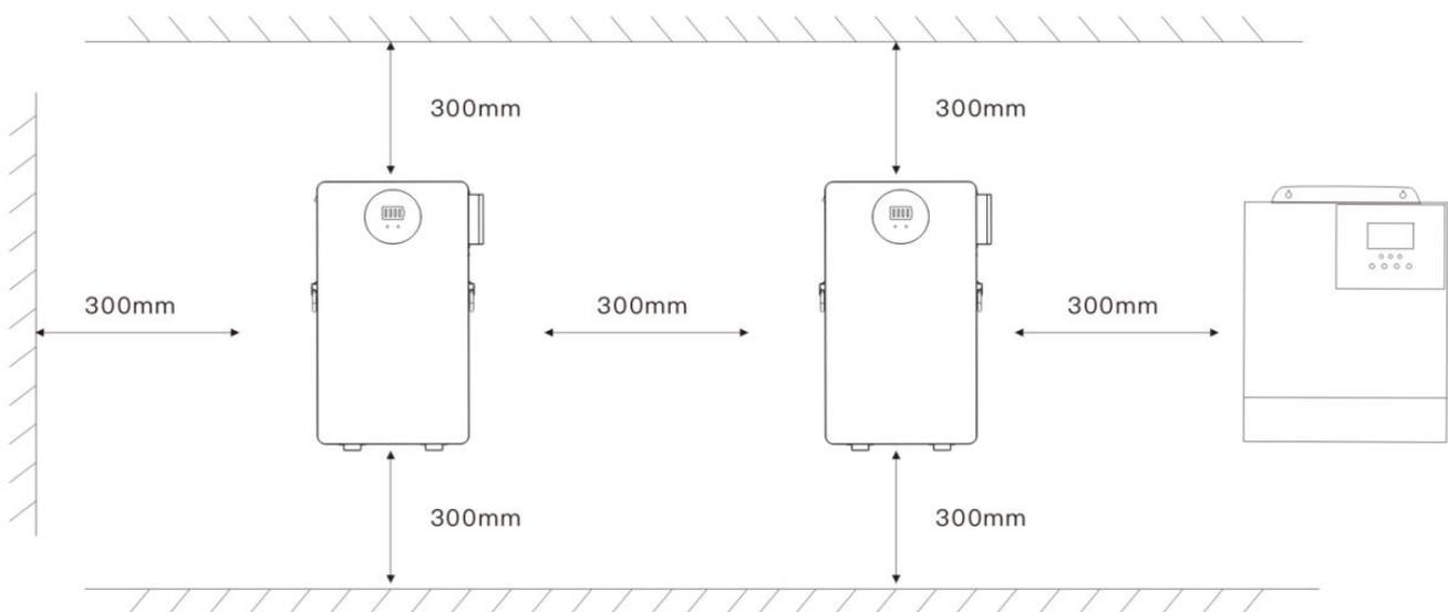
**Wall mount:** The battery should be placed in the right position first, and the installation site should be smooth and the wall should be solid, and the device is 300mm away from the ground, the distance between the batteries should be greater than 300mm.
