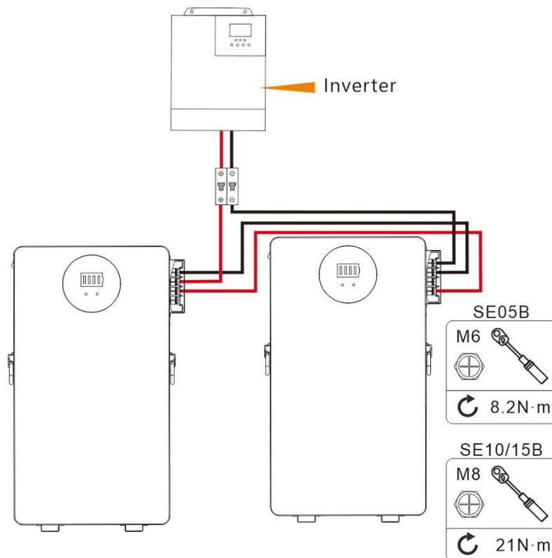
If multiple batteries are used in parallel, bus bar is required
